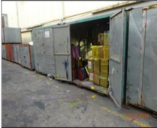
External photo(s) of the production unit(s) NC_12.4_The empty can of paint was not stored in the secondary containment.JPG
