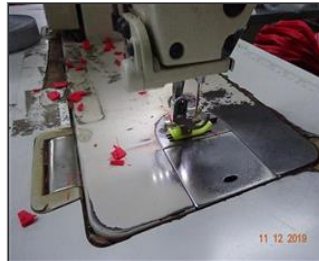
External photo(s) of the production unit(s) Needle guard was installed.JPG
